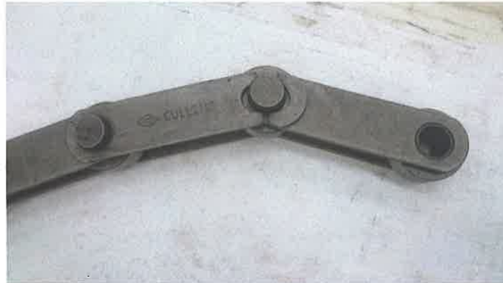
Photo. 4 – Mode of failure (ST628 - 50,000lbs)
